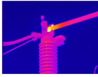
Thermographers have long used temperature differentials or Delta T measurements as a means of prioritizing electrical and mechanical exceptions. Typically, Delta T values are calculated by comparing the temperature of an exception to similar components under similar load or
