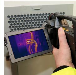
As no material is 100% transmissive to infrared energy, all infrared windows will qualitatively and quantitatively attenuate the infrared energy passing through the window. While it is useful to know the transmittance of the window's optical material, there are other important factors to be considered. It should be noted that there is no way to compensate for any of the common error sources listed below.
