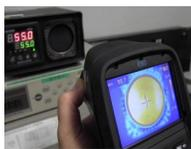
In order to check infrared radiometer calibration, you will need at least two targets, each with a known temperature and emittance. A
