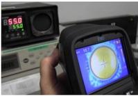
Infrared radiometers must be within calibration in order to accurately measure temperatures. Traditionally, thermographers periodically send their equipment to the manufacturer for calibration. For some, this process can take several weeks and can be rather expensive.
